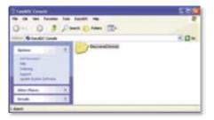
Double-click the Discovered Devices folder. The Discovered Devices screen appears showing each discovered component of the EasyADC System and its IP address.
