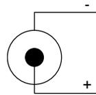
Figure 3 - Power Supply Polarity
