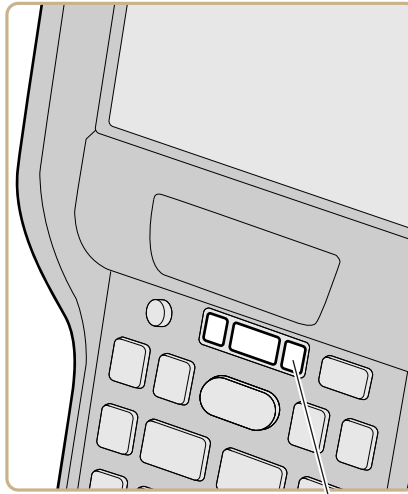
Battery status LED
