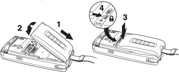
Note: The terminal does not power ON unless the battery is locked A.
