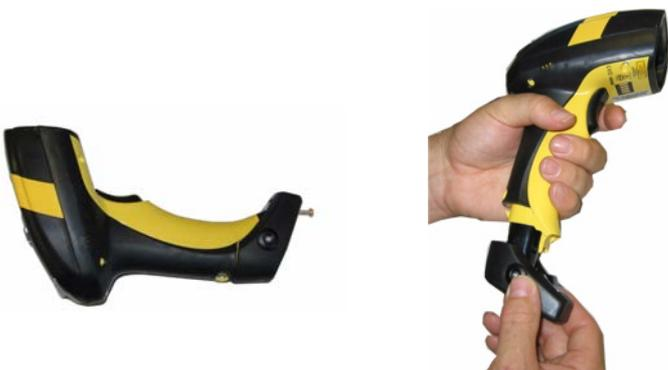
2. Insert the new battery pack containing the Magnet (included with the kit) into the reader handle. Tighten the screw to secure.
