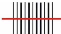
PowerScan™ PM8300-DK provides an aiming system. If enabled, a partial trigger press produces a red spot, which should be aimed over the code center to get the best reading performance, see #1 in the figure above. By completely pressing the trigger the scan line appears to start the code scanning, see #2.
