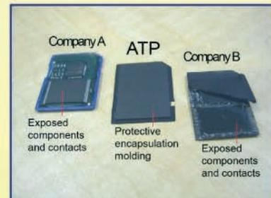
A special protective layer provides solid protection
