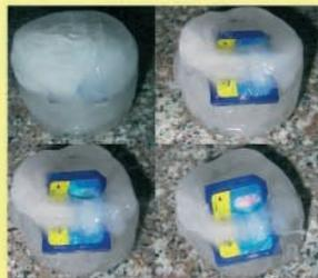
ATP SD Card in a block of ice
