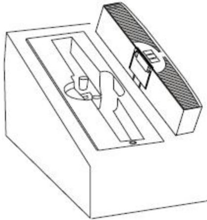
Caution! It is important that battery packs are inserted into the charging pocket correctly. Inserting the battery incorrectly could result in damage to the battery pack or the charger.
