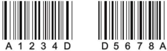
Select **Require** to prevent the scanner from decoding a single “D” Codabar symbol without its companion. This selection has no effect on Codabar symbols without Stop/Start D characters.
