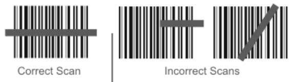
Holding the beam aperture approximately 3 – 12 inches away from the bar code, aim the scan aperture toward the selected bar code. Refer to the bar code reader engine type in *Decode Zones* later in this guide for recommended decode ranges.
