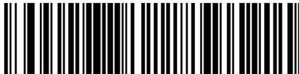
When Supplemental User-Programmable option is selected from Decode UPC/EAN Supplementals, select **User-Programmable Supplemental 2** to set the 3-digit prefix. Then select the 3 digits using the [Keypad Number Symbols](#) (page 6-91).
