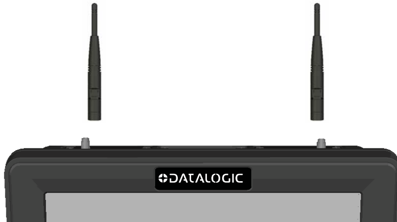
Figure 11 – Mounting the Antennas
