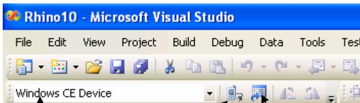
Target Device    Connect To Device    Device Options
