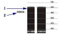
**Media Sensor Profile (Figure 29)** The media sensor readings are shown as bars and flat areas on the sensor profile. The bars (1) indicate gaps between labels (the web), and the low areas (2) indicate where labels are located. If you compare the sensor profile printout to a blank length of your media, the bars should be the same distance apart as the gaps on the media. If the distances are not the same, the printer may be having difficulty determining where the gaps are located.
