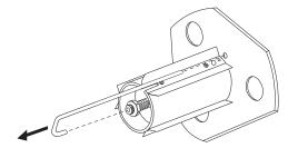
**15.** If you are using a core, slide it onto the rewind spindle until it is flush against the guide plate.
