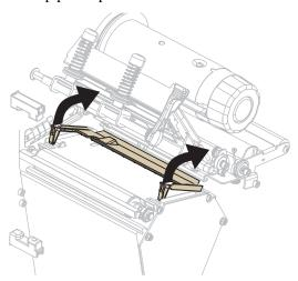
**5.** Remove the snap plate from the printer.
