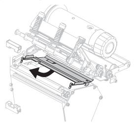
**6.** Using the swab from the Preventive Maintenance Kit (part number 47362), clean the back of the snap plate. In place of the Preventive Maintenance Kit, you may use a clean swab or soft cloth dipped in a solution of isopropyl alcohol (minimum 90%) and deionized water (maximum 10%). Allow the solvent to evaporate.
