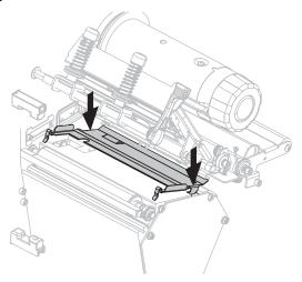
**8.** Press down on the loops to lock the snap plate into place.
