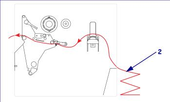
**a.** Slide out and, if applicable, flip down the media supply guide.
