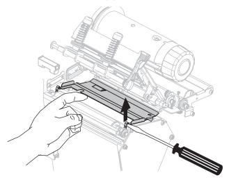
**5.** Remove the snap plate from the printer.
