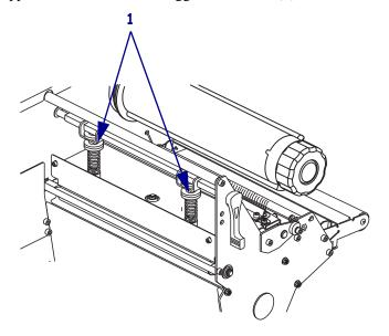
**4.** Some media types require higher pressure to print well. For these media types, increase or decrease pressure using the lower knurled nuts (1) until the left and right edges of the printed area are equally dark.
