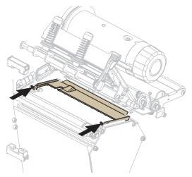
**4.** Rotate the front of the snap plate upward.
