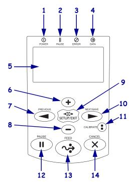
Figure 3 • Location of Control Panel Buttons and Lights
