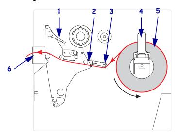
Figure 9 • Media Loaded in Cutter Mode
