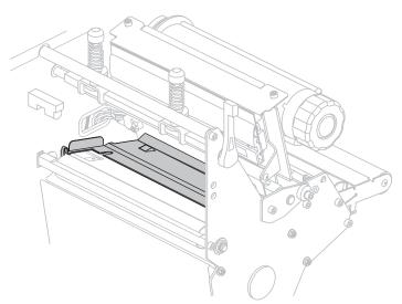
Figure 20 • Snap Plate Location
