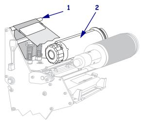
**10.** Wind the ribbon leader and attached ribbon counterclockwise around the ribbon take-up spindle.
