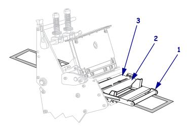
**12.** Push the media forward until it passes under the printhead assembly (**1**), under the snap plate (**2**), and then over the platen roller (**3**).
