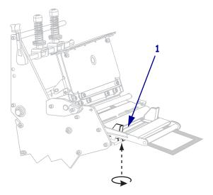
**21.** Push down the printhead assembly (1), and then rotate the printhead-open lever (2) clockwise until it locks into place.
