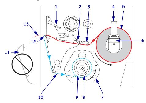
Figure 8 • Media Loaded in Peel-Off Mode
