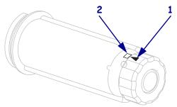
**2.** Align the segments of the ribbon supply spindle.
