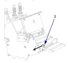
**7.** If your printer includes a media dancer assembly (1), thread the media under the media dancer assembly roller. For all printers, thread the media under the media guide roller (2) and then the upper media sensor (3).
