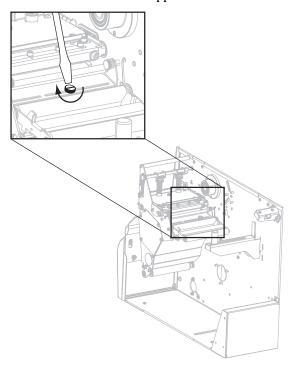
**6.** Adjust the lower media sensor to match the new position of the upper media sensor. See *Lower Media Sensor* on page 79.
