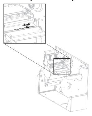
**5.** Tighten the adjustment screw to secure the upper media sensor in its new position.
