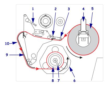
Figure 10 • Media Loaded in Rewind Mode
