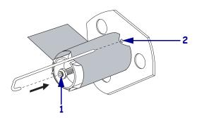
18. Rotate the spindle counterclockwise several turns to wind the media liner over the hook and remove any slack.
