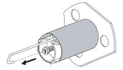
**3.** Slide the media or liner off of the rewind spindle.
